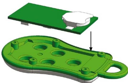
Put the electronic card back in its housing.
