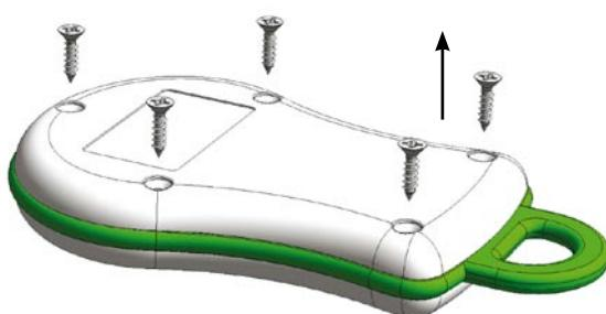
Unscrew the 5 screws then lift up the cover.
