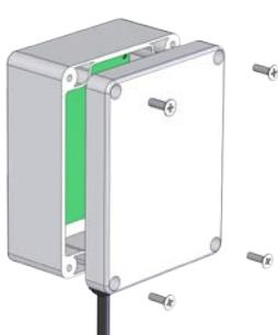
4a) Unscrew the four screws and remove the lid from the controller.
