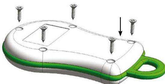
Put the cover back in place then screw in the 5 screws.
